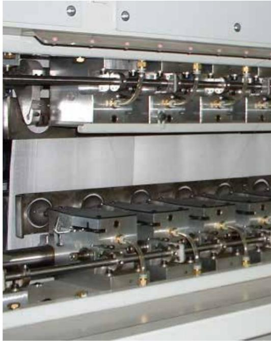
Each needle is driven by an independent sewing head, strong penetrability;
