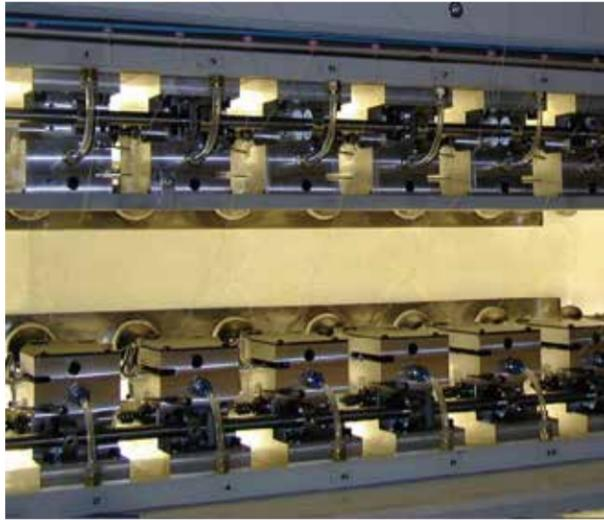
Unique vertical feeding method in the world, needle rows place can moveable, jumbo rotary hook multi needle quilting machine, some patterns can be replaced without needle layout.
