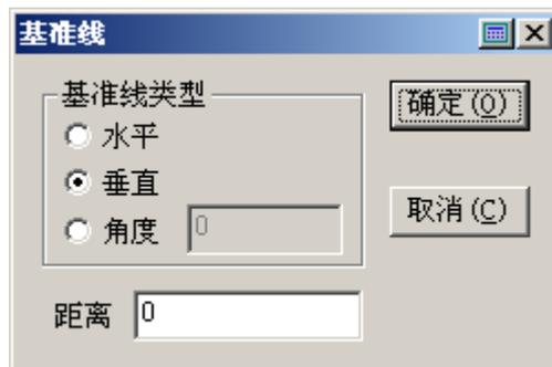
3. 复制基准线: 按住 Ctrl 键, 用
